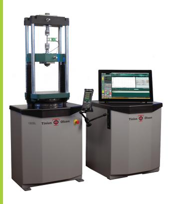
he Model 150SL is designed for tension, compression, flexure and shear strength testing on materials and assemblies. The robust design incorporates quality materials and components to ensure that our reputation for superior system performance, ease of use and longevity is maintained.
