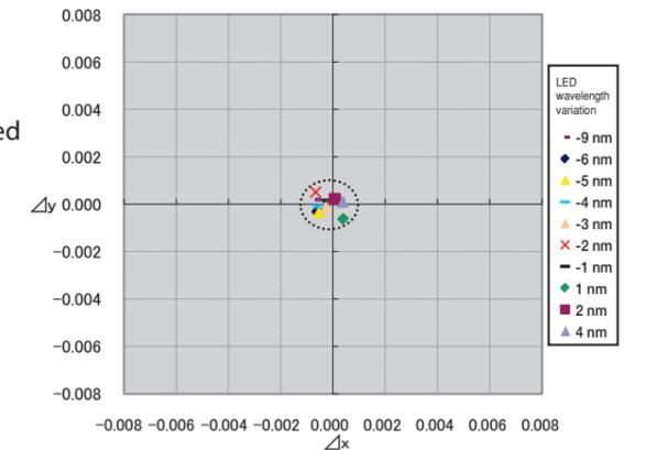
\*Errors (differences from true values) for white LEDs with different peak wavelengths when measured using CA-310. User calibration to standard LED performed.
