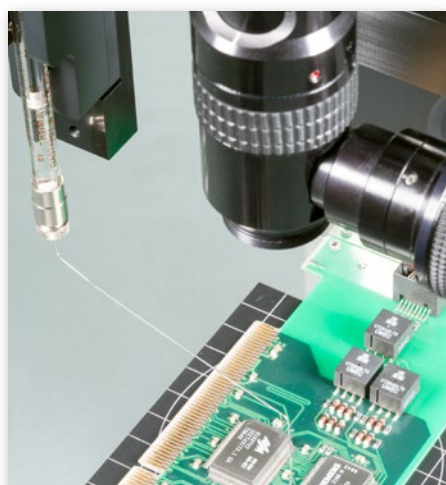
Topview Video System TVS for contact angle measurements in topview
