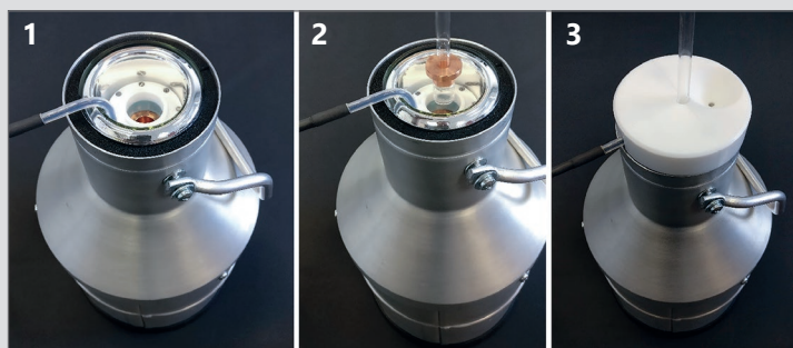
Figure 5 The use of a cryoTune: the cryoTune is placed inside the dewar (1). The sample cell is then placed into the cryoTune (2). Finally, the dewar is closed with the special isolation cover (3).
